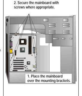
Ensure that your case has an I/O template that supports the I/O ports and expansion slots on your mainboard.
