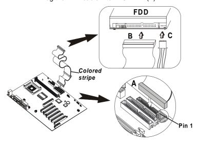
Note: The ribbon cable connectors are keyed so that they can only be installed correctly on the device connector. If the connector is not keyed, make sure that you match the pin-1 side of the cable connector with the pin-1 side of the device connector. Each connector has the pin-1 side clearly marked. The pin-1 side of each ribbon cable is always marked with a colored stripe on the cable.
