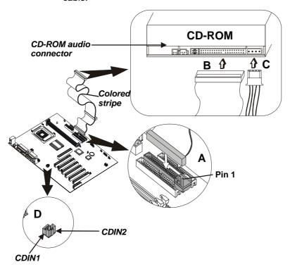
**Note:** The ribbon cable connectors are keyed so that they can only be installed correctly on the device connector. If the connector is not keyed, make sure that you match the pin-1 side of the cable connector with the pin-1 side of the device connector. Each connector has the pin-1 side clearly marked. The pin-1 side of each ribbon cable is always marked with a colored stripe on the cable.
