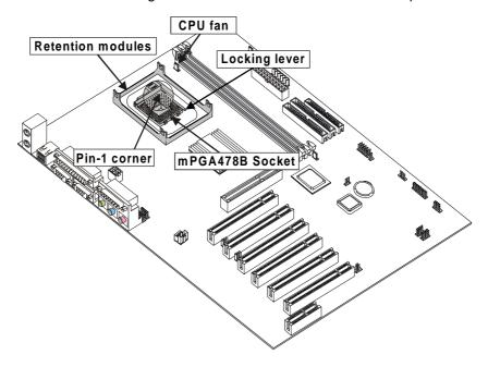
**Note:** The pin-1 corner is marked with an arrow **▼**
