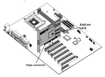
3. Secure the metal bracket of the card to the system case with a screw.
