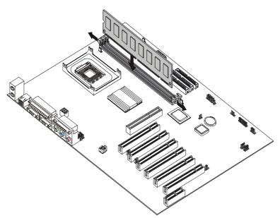
Align the memory module with the slot. The DIMM slots are keyed with notches and the DIMMs are keyed with cutouts so that they can only be installed correctly. Check that the cutouts on the DIMM module edge connector match the notches in the DIMM slot:
