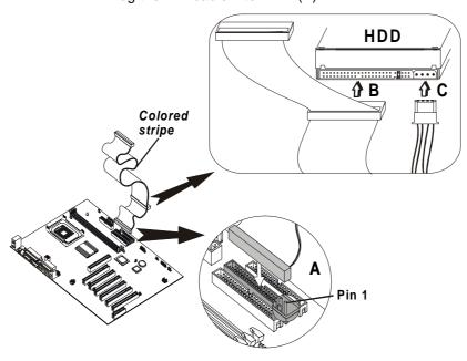
Note: The ribbon cable connectors are keyed so that they can only be installed correctly on the device connector. If the connector is not keyed, make sure that you match the pin-1 side of the cable connector with the pin-1 side of the device connector. Each connector has the pin-1 side clearly marked. The pin-1 side of each ribbon cable is always marked with a colored stripe on the cable.
