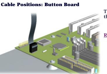
This image indicates the cable routing for connecting the Button Board to the system board.
