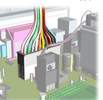
This image indicates the cable routing for the Power Supply Assembly to the system board.
