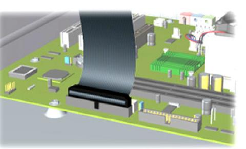
This image indicates the cable routing for connecting the Hard Drive to the system board.
