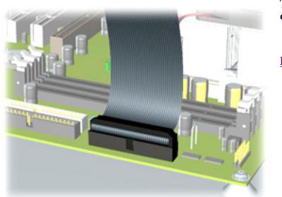
This image indicates the cable routing for connecting the Disk Drive to the system board.
