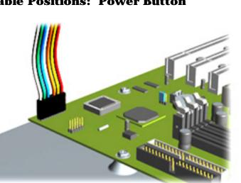
This image indicates the cable routing for connecting the Power Button to the system board.
