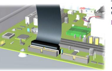
This image indicates the cable routing for connecting the CD, CD-RW, and/or DVD Drive to the system board.
