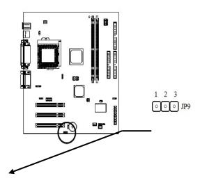
You need to clear the CMOS if you forget your system password. The procedure of clear CMOS is as following:
