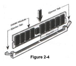
**NOTE!** When you install DIMM module fully into the DIMM socket the eject tab should be locked into the DIMM module very fimly and fit into its indention on both sides.
