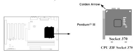
When you put the CPU into the ZIF socket. No force require to insert of the CPU, then press the level to Locate position sightly without any extra force.
