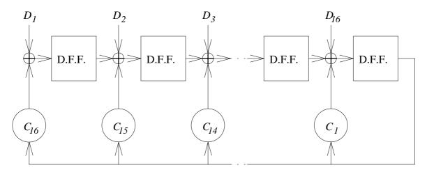
Figure 3-34 Multi-Input Signature Register (MISR)
