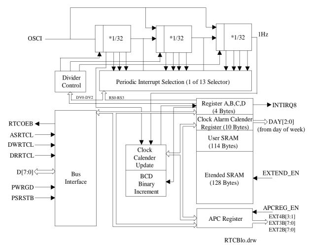
Figure 3-12 Block Diagram of RTC
