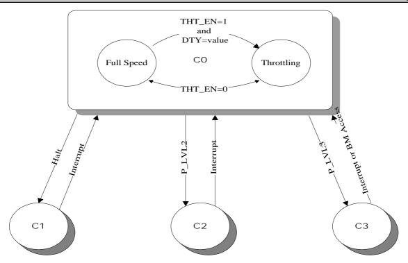
Figure 3-17 Processor Power State Diagram
