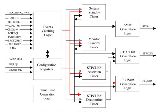
Figure 3-6 Legacy PMU Block Diagram
