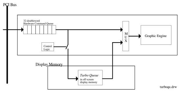
Figure 3-33 Turbo Queue Architecture
