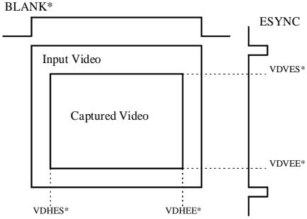
Integrated VGA Controller provides video capture windowing to select a part of input video to be captured into video frame buffer. This capture window is defined by four parameter: video data horizontal start (VDHES), video data horizontal end (VDHEE), video data vertical start (VDVES), and video data vertical end (VDVEE).
