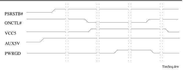
Figure 3-13 Typical Timing Sequence on the Power Control Related Signals
