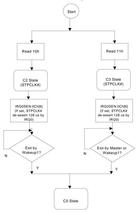
Figure 3-26 CPU Power State Flow Chart
