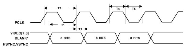
Figure 7-1 Video Timing 4, 8, 24 Bits/Pixel Modes
