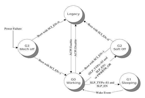
Figure 3-15 Global System State Diagram
