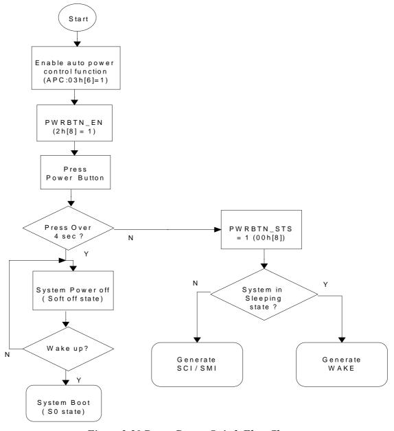
Figure 3-20 Power Button Switch Flow Chart
