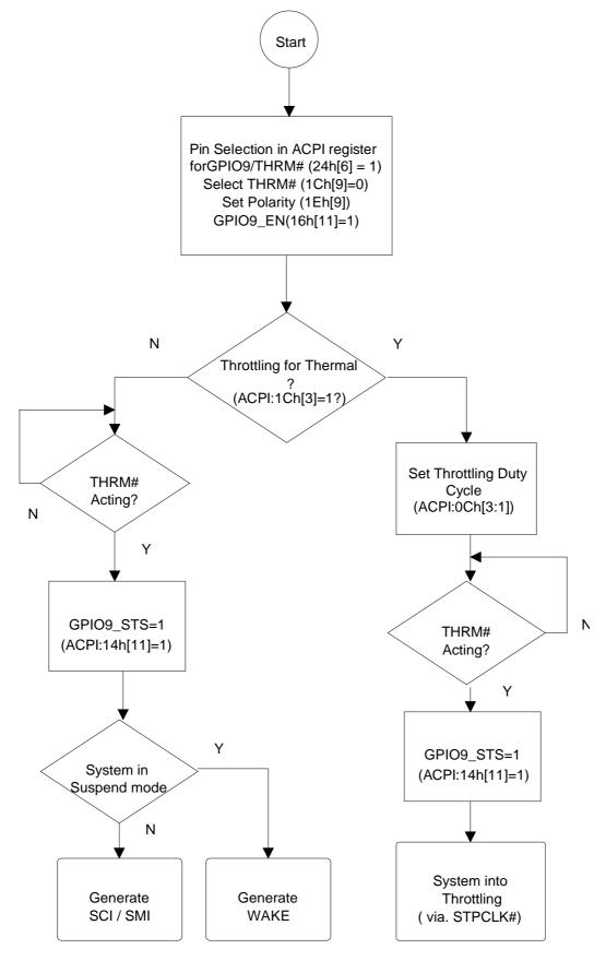
Figure 3-25 Thermal Detection Flow Chart
