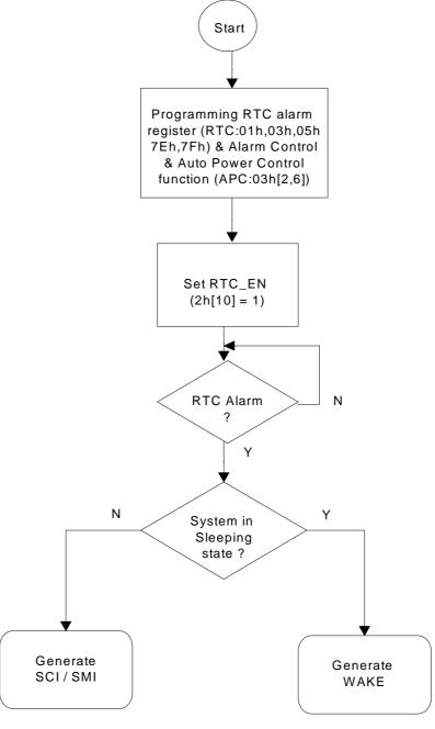
Figure 3-21 RTC Alarm Flow Chart
