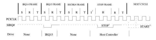
H=Host Control R=Recovery T=Turn-around S=Sample I=Idle
