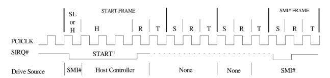
H=Host Control SL=Slave Control R=Recovery T=Turn-around S=Sample
