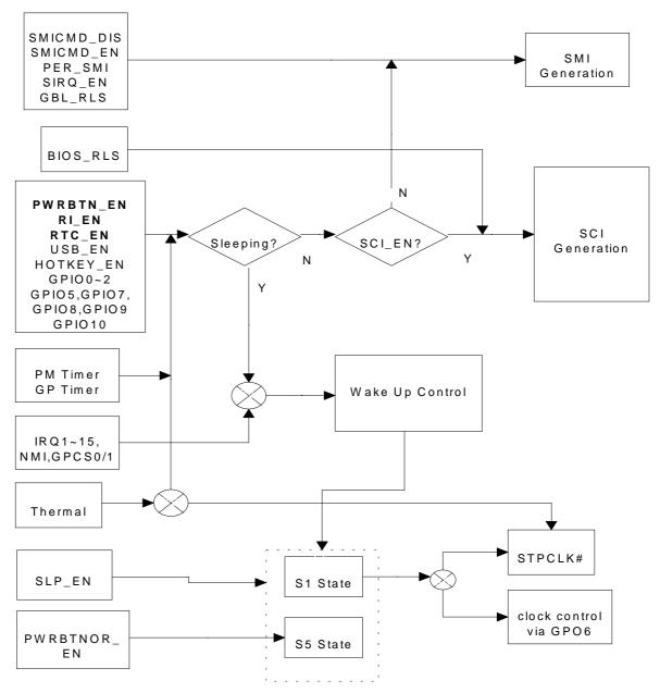
Figure 3-18 ACPI working mechanism overview
