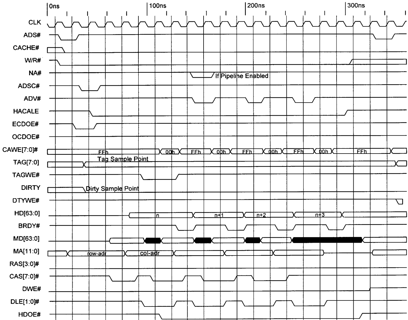
Figure 4-11 L2 Cache Read Miss Clean Burst of 8-3-3-3 (Linefill Cycle) - Sync. SRAMs
