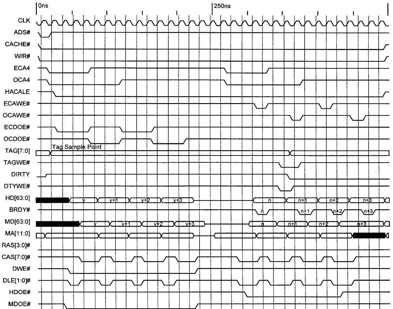
Figure 4-12 L2 Cache Read Miss Dirty Cycle - Async. SRAMs
