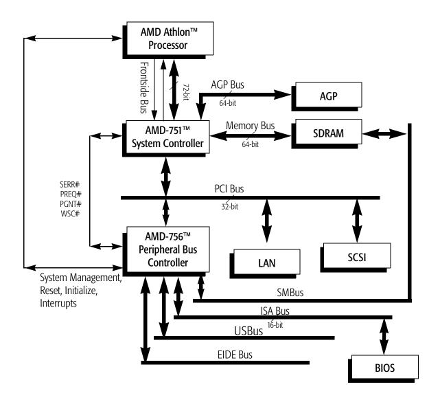
Figure 1. AMD-750™ Chipset System Block Diagram
