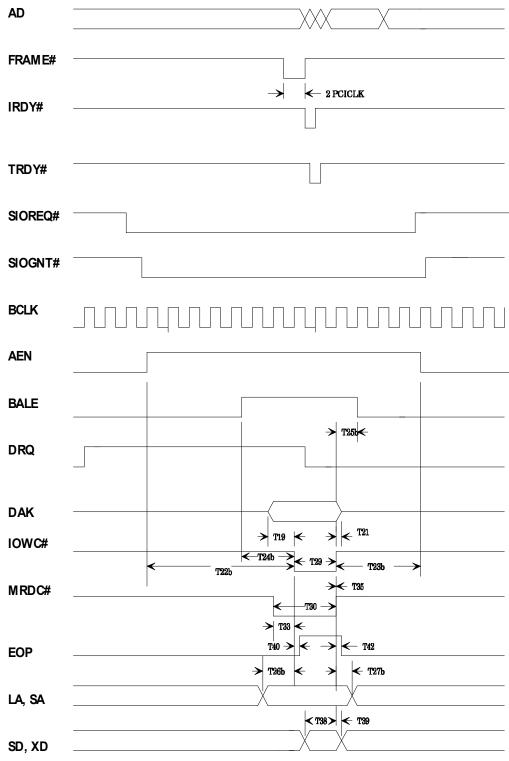
DMA cycle (IORC#, MWTC#), DMACLK = BCLK
