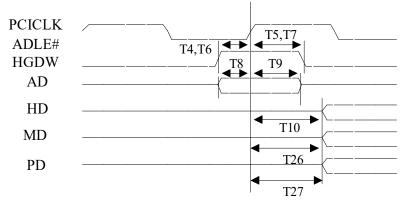
Figure 3.8 CPU Read PCI Slave Cycle
