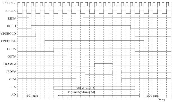
Note: HOLD,CIP# (current in progress) are internal signal
