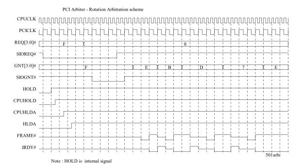
A PCI master can burst so long as the target can source/sink the data, and no other agent requests the bus. However, PCI specifies two mechanisms that cap a master's tenure in the presence of other requests, so that predictable bus acquisition latency can be achieved. One is
