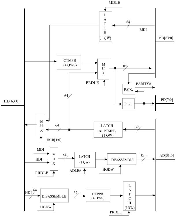
Figure 3.1 PLDB Block Diagram
