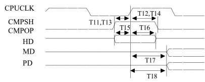
Figure 3.4 CPU Write DRAM Cycle
