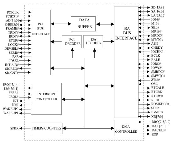
Figure 4.1 SiS85C503 Functional Block Diagram
