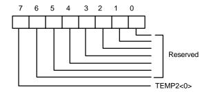
Bit 7: Temperature <0> of sensor2, which is low byte.
