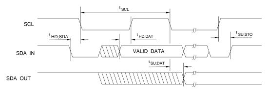
Serial Bus Timing Diagram
