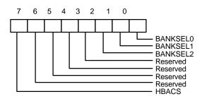
Bit 7: HBACS- High byte access. Set to 1, access Register 4Fh high byte register.
