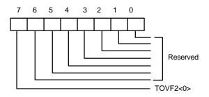
Bit 7: Read/Write - Over-temperature bit 0, which is low Byte.
