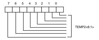
Bit 7: Temperature <8:1> of sensor 2, which is high byte.
