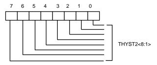
Bit 7-0: Temperature hysteresis bit 8-1, which is High Byte. The temperature default 75 degree C.
