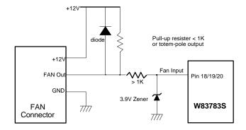
Figure 13-4. Fan with Tach Pull-Up to +12V, or Totem-Pole Putput and Zener Clamp
