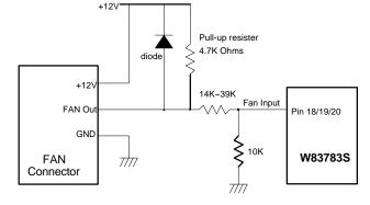
Figure 13-1. Fan with Tach Pull-Up to +5V
