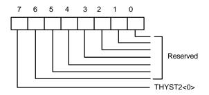
Bit 7: Temperature hysteresis bit 0, which is low Byte.
