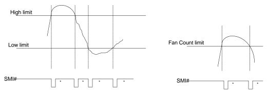
\*Interrupt Reset when Interrupt Status Registers are read
