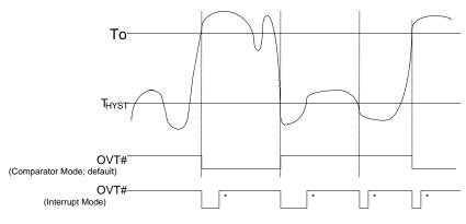
\*Interrupt Reset when Temperature 2/3 is read
