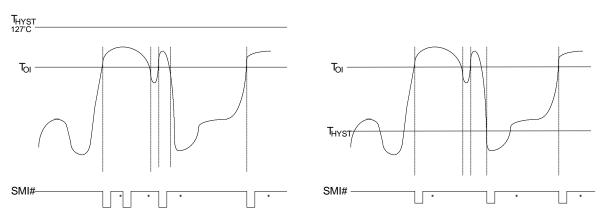
\*Interrupt Reset when Interrupt Status Registers are read
