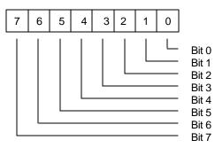
Bit 7 ~ 0: Clock base value. It specifies number of internal sampling clock pulses for a data bit. Default to be 0Ch.
