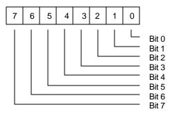
Bit 7 ~ bit 0: Access port for receiver FIFO.
