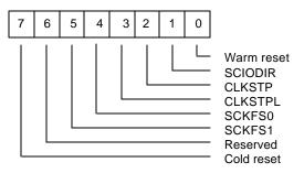
Bit 7: Cold reset. Setting "1" to this bit turns off power to Smart Card interface by pulling up SCPWR#. SCCLK is stopped, SCRST# kept low, SCIO in input mode and SCLED is inactive. ECR's SCIODIR, SCKFS1 and SCKFS0 control bits and control bits in CBR, GTR, BLH and BLL are cleared to default values. User must write a "0" to this bit to recover to normal state.
