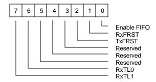
Bit 7, 6: RxTL1 and RxTL0 mean receiver FIFO active threshold level control bits. These two bits are used to set the active level for the receiver FIFO interrupt. For example, if the interrupt active level is set as 4 bytes, once there are at least 4 data characters in the receiver FIFO, an interrupt is activated to notify host to read data from FIFO. Default to be 00b.
