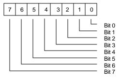
Bit 7 ~ 0: Baud rate divisor latch lower byte values. Default to be 1Fh.
