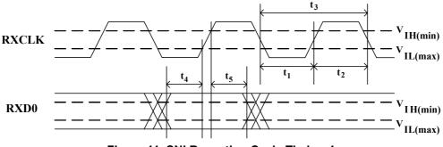
Figure 11. SNI Reception Cycle Timing-1
