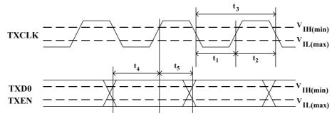
Figure 9. SNI Transmission Cycle Timing-1
