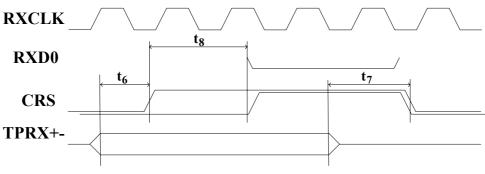
Figure 12. SNI Reception Cycle Timing-2
