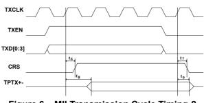
Figure 6. MII Transmission Cycle Timing-2
