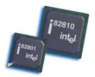
• The 82801 *I/O Controller Hub (ICH)* employs the Hub Architecture to make a direct connection from the graphics and memory to the integrated AC97 controller, the IDE controllers, dual USB ports, and PCI add-in cards.
