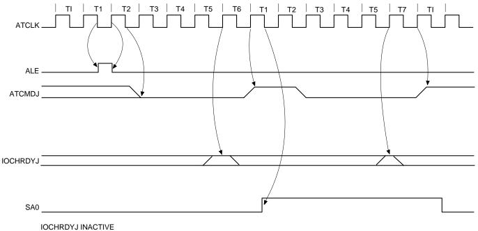
OWS INACTIVE IF IOCHRDYJ IS INACTIVE, CYCLE WILL BE ADDED AT T5. IF OWSJ IS ACTIVE AT T2,..T4, THE CYCLE WILL GO INTO T6.
