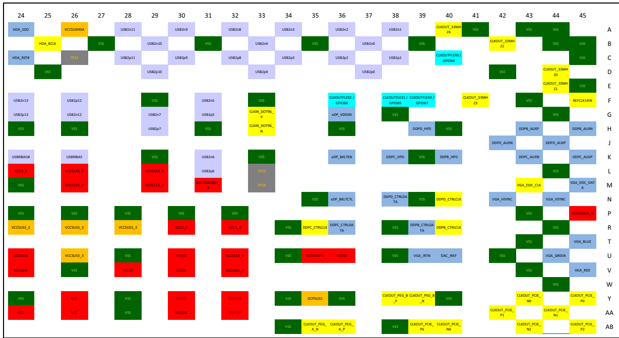
Figure 6-8. Mobile PCH Ballout (Top View - Lower Right)
