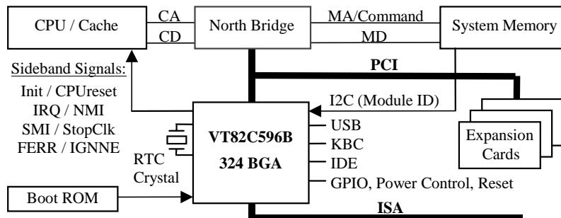
**Figure 1. PC System Configuration Using the VT82C596B**
