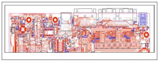
Figure 6. Top Signal Layer after the Ground Fill Near the I/O Layer
