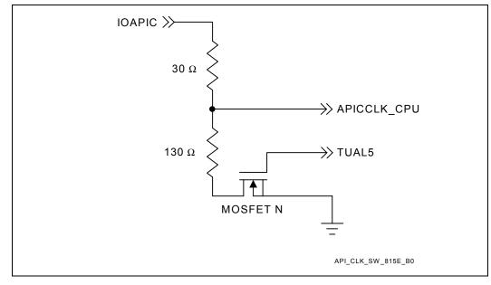
NOTE: The 30  $\Omega$  resistor represents the series resistor typically used in connecting the APIC clock to the processor.
