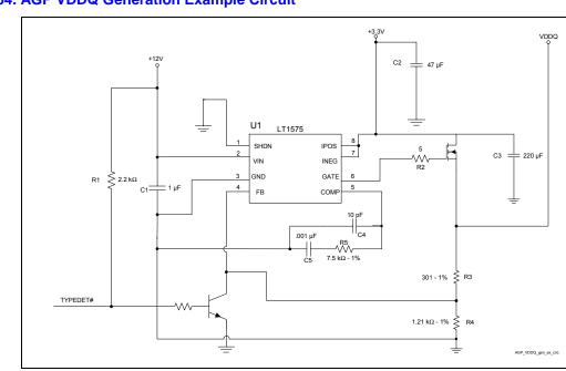
Figure 54. AGP VDDQ Generation Example Circuit
