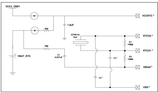
Figure 107. Intel<sup>®</sup> ICH2 Oscillator Circuitry
