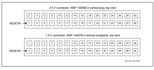
*Caution:* The Pentium III processor (CPUID=068xh) and Celeron processor (CPUID=068xh) require an intarget probe (ITP) compatible with 1.5 V signal levels on the TAP. Previous ITPs were designed to work with higher voltages and may damage the processor if connected to any of these specified processors.
