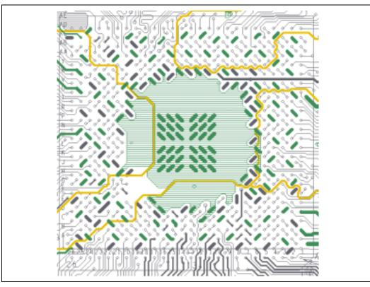
Yellow lines in Figure 47 show layer two plane splits. (Printed versions of this document will show the layer two plane splits in the left-side, bottom, right-side, and upper right-side quadrants
