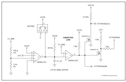
**NOTE:** the diode is included so that repeated pressing of the reset or power button does not cause the capacitor to build up enough charge to circumvent the 20 ms delay.
