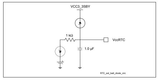
A standby power supply should be used in a desktop system, to provide continuous power to the RTC when available, which will significantly increase the RTC battery life and, thereby, the RTC accuracy.
