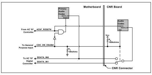
**NOTE:** Figure 69 shows the circuitry required on the motherboard to support a two-codec down configuration. This circuitry disables the codec on a single codec CNR. Notice that in this configuration the resistor,  $R_B$ , has been changed to 100 k $\Omega$ .
