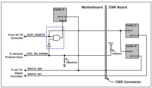
As shown in Figure 67, when a single codec is located on the motherboard, the resistor  $R_A$  and the circuitry (AND and NOT gates) shown inside the dashed box must be implemented, on the motherboard. This circuitry is required to disable the motherboard codec when a CNR is installed which contains two AC '97 codecs (or a single AC '97 codec which must be the primary codec on the AC-link).
