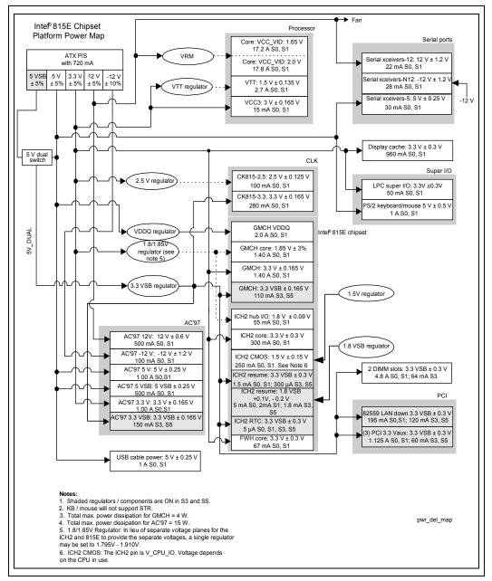
In addition to the power planes provided by the ATX power supply, an *instantly available* 815EP universal platform (using *Suspend-to-RAM*) requires six power planes to be generated on the board. The requirements for each power plane are documented in this section. In addition to on-board voltage regulators, the CRB will have a *5V Dual Switch*.
