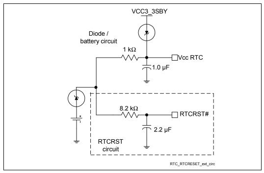
This RTCRST# circuit is combined with the diode circuit (see Figure 81), which allows the RTC well to be powered by the battery when system power is unavailable. Figure 81shows an example of this circuitry when used in conjunction with the external diode circuit.
