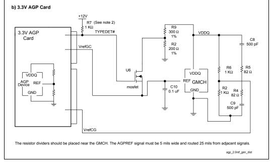
The flexible VREF divider shown in Figure 55 uses a FET switch to switch between the locally generated VREF (for 3.3 V add-in cards) and the source-generated VREF (for 1.5 V add-in cards).
